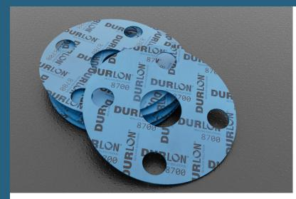
Durlon<sup>®</sup> 8700 is a high performance gasket material for use in processes requiring a neoprene (CR) bonded sheet and has excellent hand and die cutting characteristics. This product has excellent resistance to oils, non-aromatic solvents and many refrigerants.
