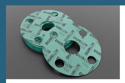
Durlon® 7925 is are an economy grade general service gasket sheet material made with NBR (Nitrile Butadiene Rubber) binder for mild service in piping and equipment with applications in steam, hydrocarbons and refrigerants and an alternative when temperature and pressure conditions are below 500°F (260°C) and 1,200 psig (See PxT chart below for validation).
